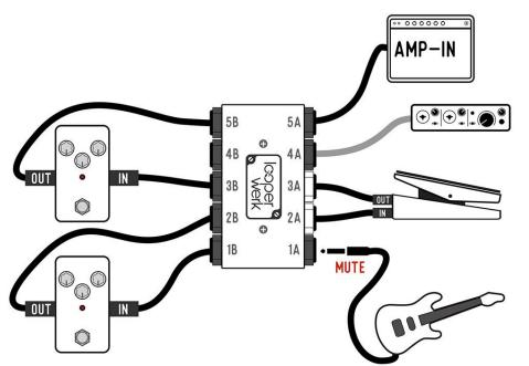
**Channel 1: Mute** - If the outer socket 1A is not used, the input of the pedalboard is muted.
